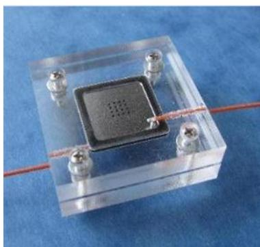
Figure 7: Fluidic test cell (closed type) for liquid flow through.
