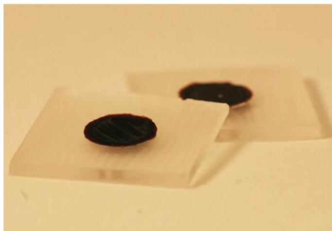
**Figure 4: Photo of the transferred porous silicon membrane onto OSTE(+) chips.**
