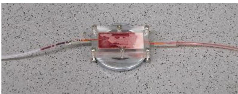
**Figure 17: Blood filter module under test. Whole blood is injected through the left hand side tubing, and the filtered plasma exits on the right hand side.**
