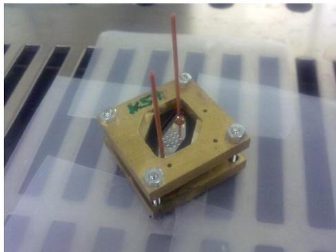
**Figure 9: Fluidic test cell (glass window type) for liquid flow through/bypass, with brass package.**
