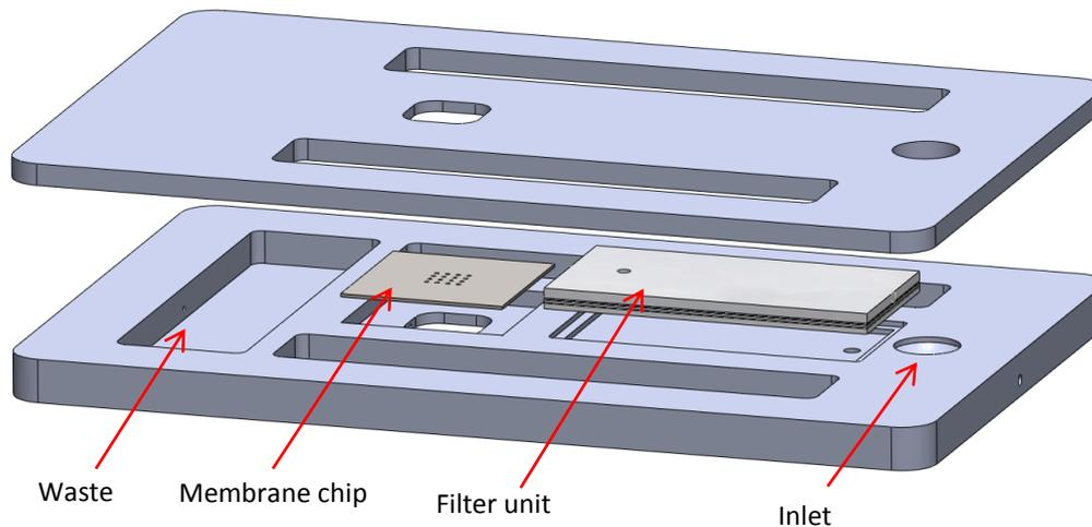
**Figure 10: Overview of fluidic cartridge, showing the four main modules: Inlet reservoir, blood filter, chip compartment for the pSi chip, waste reservoir.**
