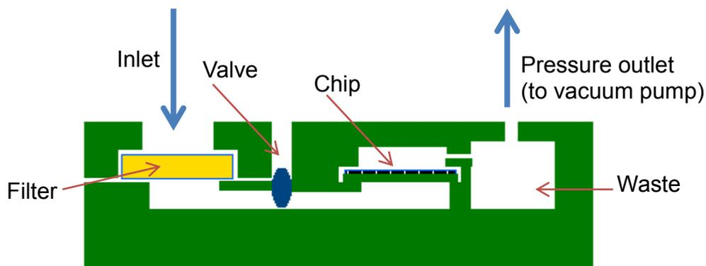
**Figure 1: Schematic of the fluidic system (disposable cartridge).** The blood sample is filtered before passing through the sensor membrane chip. A hydraulic valve seals off the chip chamber during measurements. Waste fluids are retained in the cartridge.
