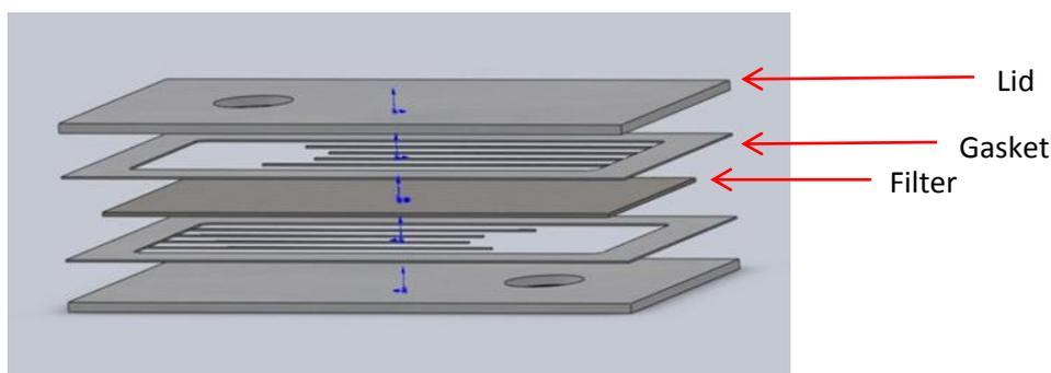
**Figure 13: Blood filter unit composed of five layers. The filter membrane in the middle is embedded by channel gaskets and top/bottom lids. The channel gaskets distributes the flow over the filter membrane are while maintaining a minimal volume between membrane and the inlet/outlet.**
