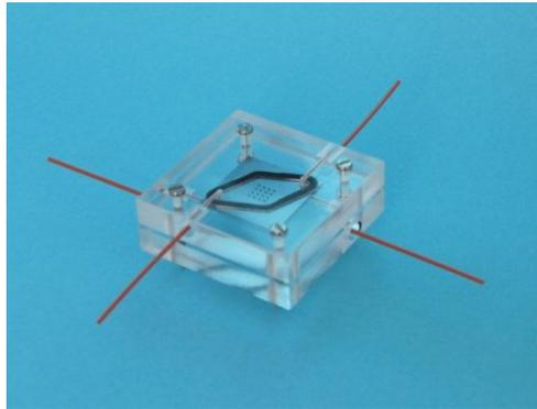
**Figure 8: Fluidic test cell (closed type) for liquid flow bypass and/or through, with minimized cell volume.**
