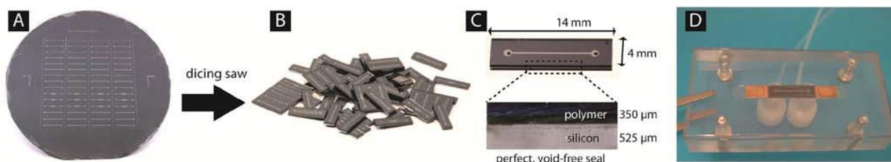
**Figure 2: Pictures from OSTE processing and pressure test set-up: (A) bonded layer of OSTE on a silicon wafer; (B) diced chips; (C) 1st demonstrator chips, demonstrating void-free seals; and (D) the “1st demonstrator” chip in the holder used for pressure tests.**
