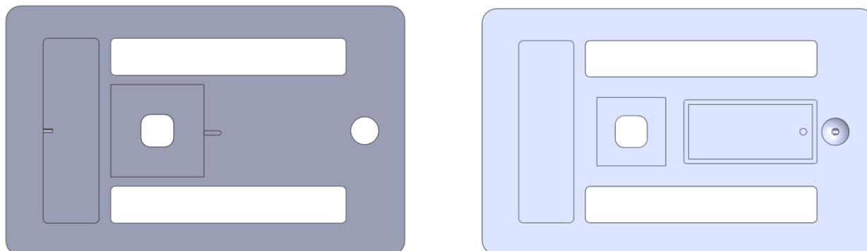
**Figure 14: Cartridge design details. Left: Upper part (lid) seen from below. Right: Bottom part (base) seen from above.**
