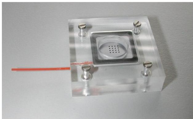
Figure 6: Fluidic test cell (open type) for accessing the membranes from one side.
