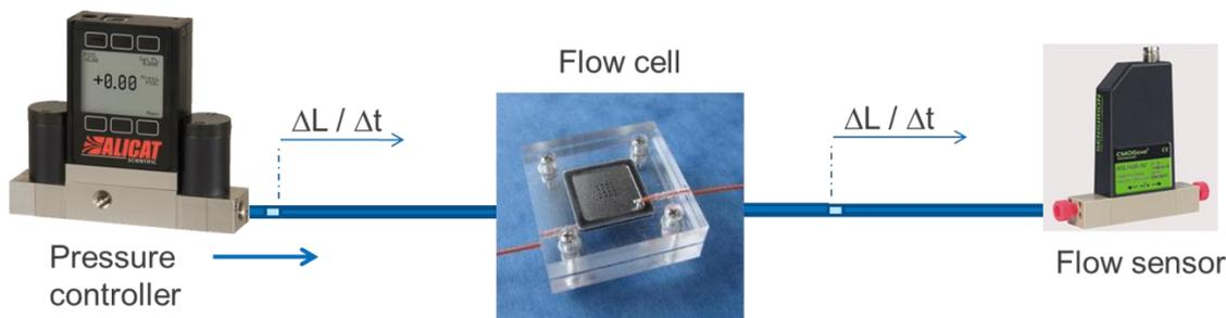
Figure 15: Test setup for flow-through characterization of fluidic components.
