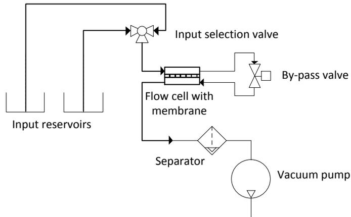
**Figure 18: Flow diagram of semi-automated microfluidic setup for biological assay**
