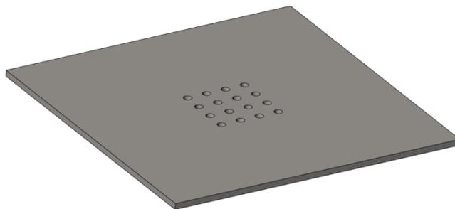
Figure 5: Porous silicon membrane array chip (CAD model).
