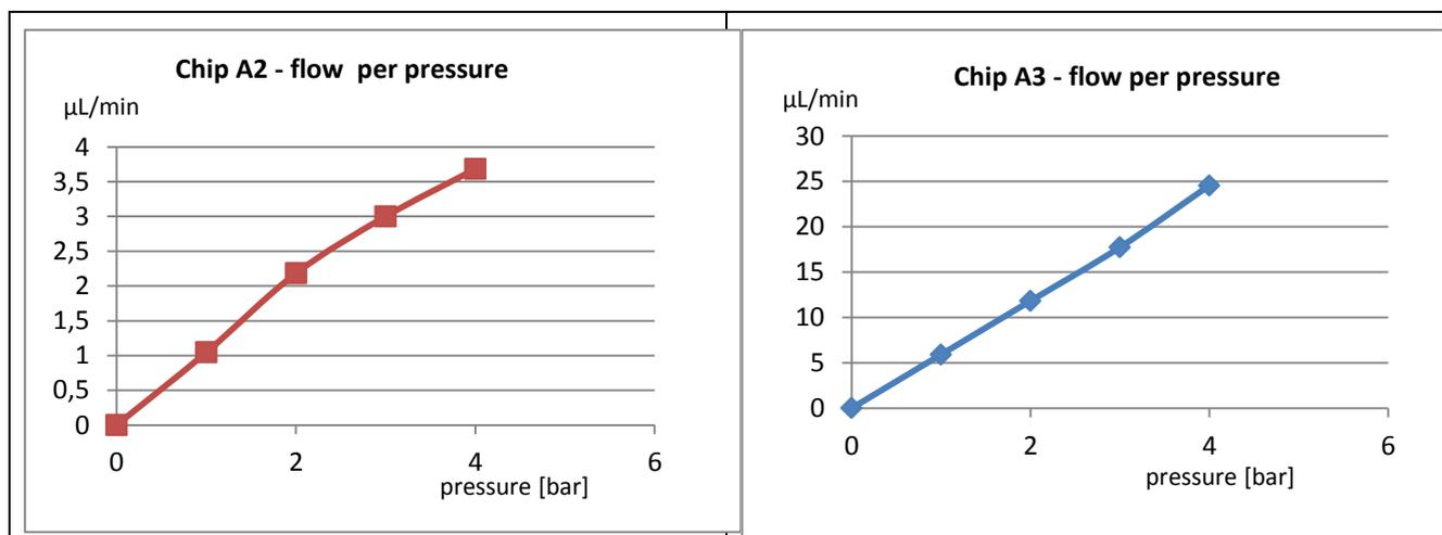
Figure 16: Flow as function of pressure through two “A” series membranes.
